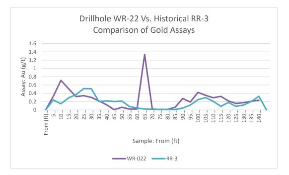
Figure 12.1. 2021 drillhole WR-22 vs. historical hole RR-3: comparison of gold assays
