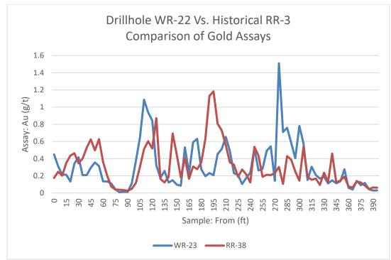
Figure 12.2. 2021 drillhole WR-23 vs. historical RR-38: comparison of gold assays
