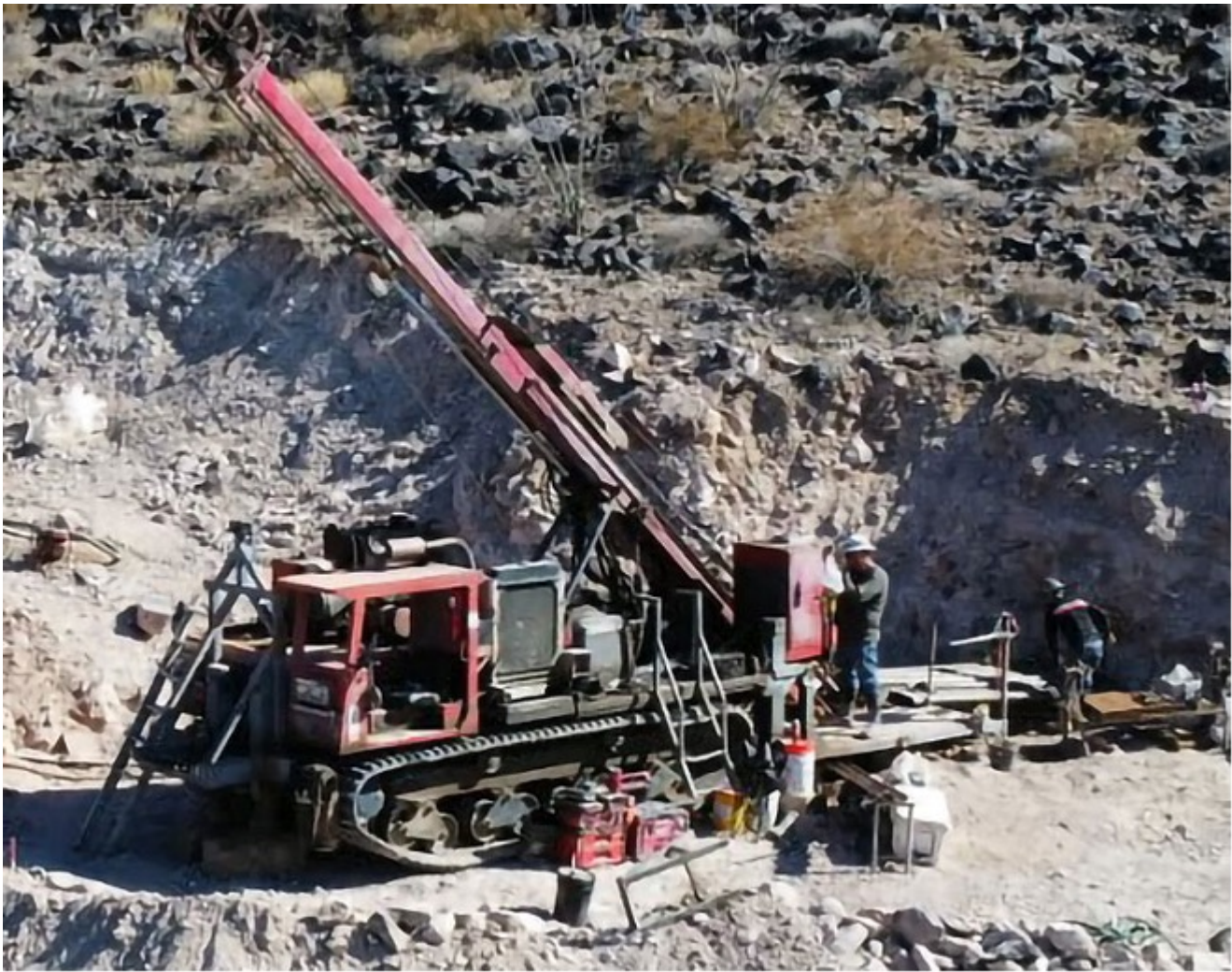
Figure 2. File Photo of the Titan Core Drilling Rig that is being used at the Eldorado Property
